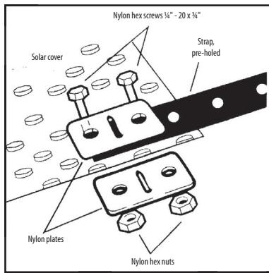
When you install the attachment kits, it must be at an equal distance amongst them. The length of the attachment must be adjusted in accordance to the shape of the pool.
