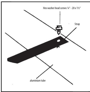
Drill holes in the aluminium tube to fix the straps which are attached to solar cover.
